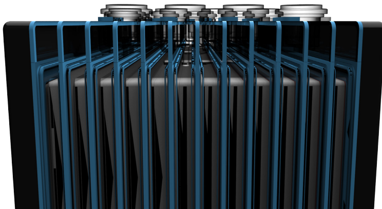
Figure 15: Mechanical design of a 24V Silicon Joule battery. Individual cells are hermetically sealed to their neighbors with silicon wafer current collectors. As there is no shared headspace for hydrogen accumulation, hydrogen explosions should be less likely to occur during its operation.
