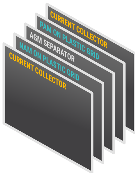
Figure 4: Cell construction of the Silicon Joule battery. Commercial positive and negative active materials are pasted onto plastic grids for mechanical support. The pasted grids are isolated with an absorbed-glass-mat separator and sandwiched between current collectors.
