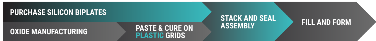
Figure 13: Comparison of typical AGM VRLA and Gridtential bipolar battery manufacturing. Manufacturers of Silicon Joule battery can purchase silicon biplates and eliminate grid casting. A simple stack-and-seal assembly step replaces welding, boxing, and sealing steps.
