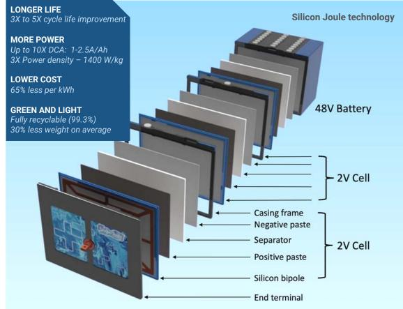
Simplified battery construction is compatible with existing manufacturing infrastructure
