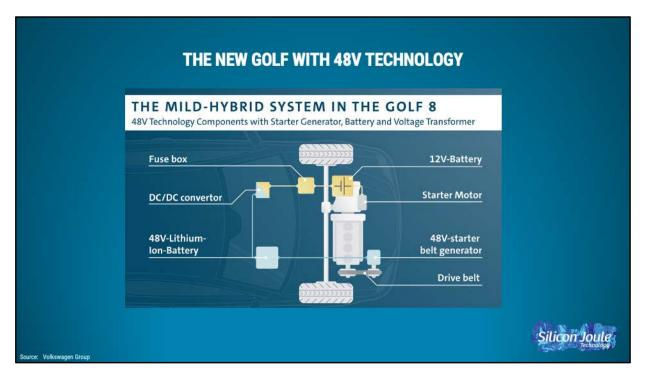
Shifting from high voltage to low voltage hybrids, here is a schematic of the mild hybrid being delivered in VW's most popular passenger car in Germany, the Golf, which aids the small, gas sipping, 1 and 1.5 liter engines in acceleration and overall efficiency.
