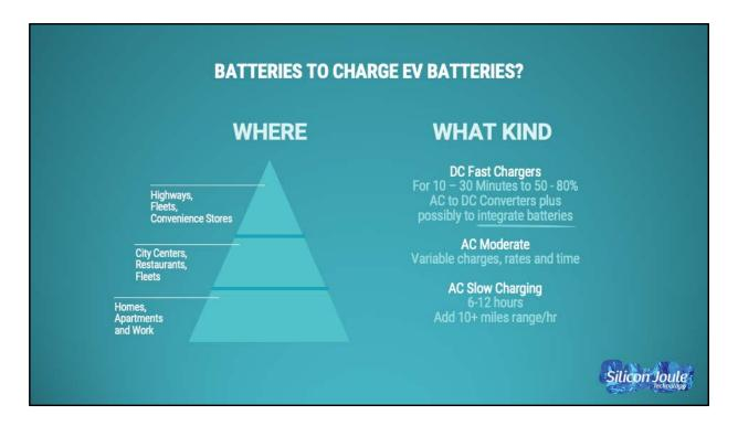
Let's talk battery chargers, both because of their role in building confidence in EV drivers, and also because applications are emerging which may include batteries to help with the fast DC charging stations evolving in many countries.
